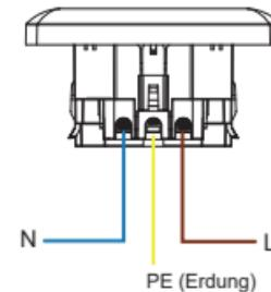
Connect the 3 wire cable to the terminals according to the figure above and fix each with the corresponding screw. (Lock the ground terminal screws in front of the socket)
