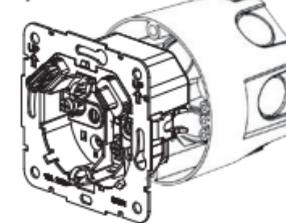
Fix the single socket outlet in a flush mount box using either claws or the mounting frame if you choose the latter method, remove the claws before mounting!
