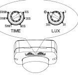
When testing in daylight, please turn LUX knob to (SUN) position, otherwise the sensor lamp could not work! If the lamp is more than 60W, the distance between lamp and sensor should be 60 cm at least.
